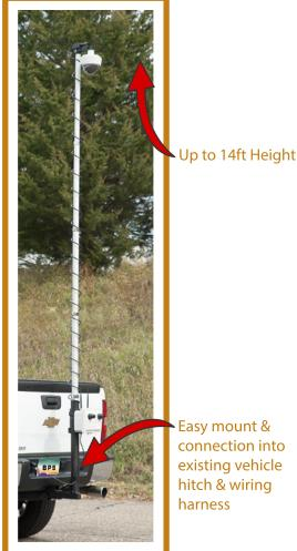
Easy mount & connection into existing vehicle hitch & wiring
